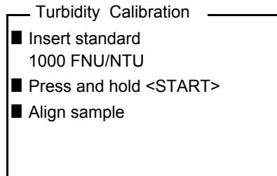
5 Insert the cell with the displayed calibration standard (here e.g. 1000 FNU/NTU) in the cell shaft (see section 4.2).
