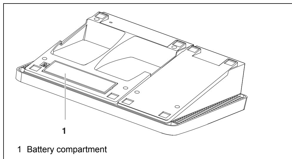
1. Open the battery compartment (1) on the underside of the meter.
